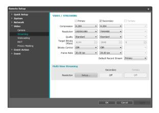
Primary/Secondary/Tertiary: Multistreaming is supported (priority: Primary > Secondary > Tertiary). Enable/disable streaming use. The lower stream settings may change depending on higher stream settings. The tertiary stream may not be available depending on higher stream settings (refer to the table below).
